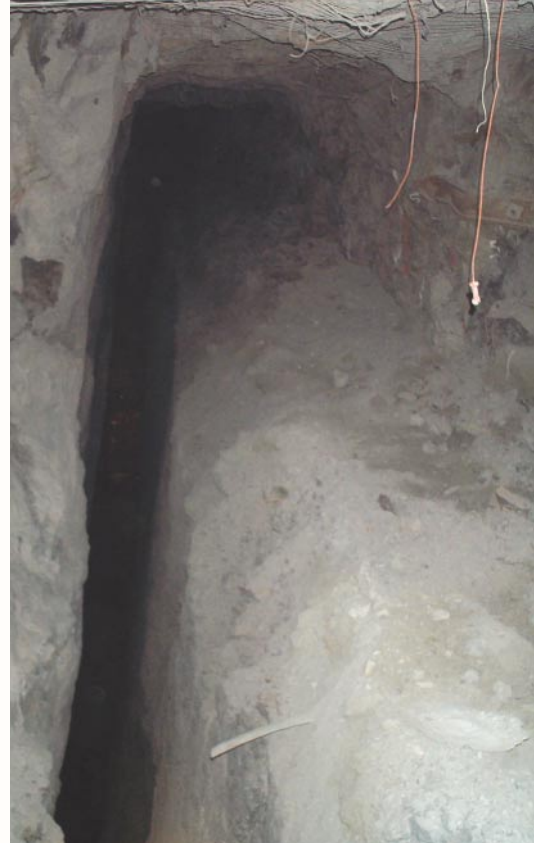
Narrow vein, longhole stope at Gympie Eldorado Mine, Gympie, Queensland (photograph by permission of Gympie Eldorado Mines). The drive is 2.5m wide and the stope is 0.9m wide.
