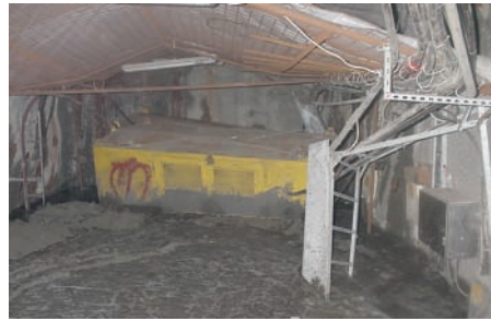
Figure 1 Property damage caused by a bulkhead failure (transformer)
