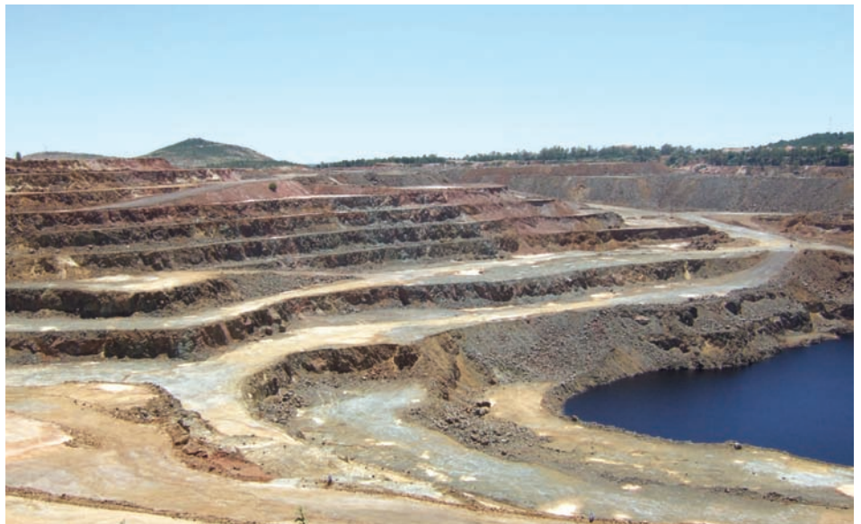
Open pit benches ready for blasting.
